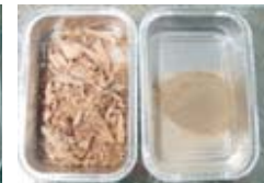
Wood: 50ml steel jar / 20 mm steel ball 200 Micron after 90 seconds
