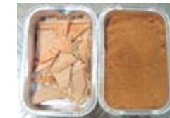
Linoleum: 50ml steel jar / 20 mm steel ball 200 micron after 60 seconds
