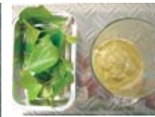
Leaves: Micro vial adapter plate / Micro vials / 3mm tungsten carbide bead per vial. Completely homogenized
